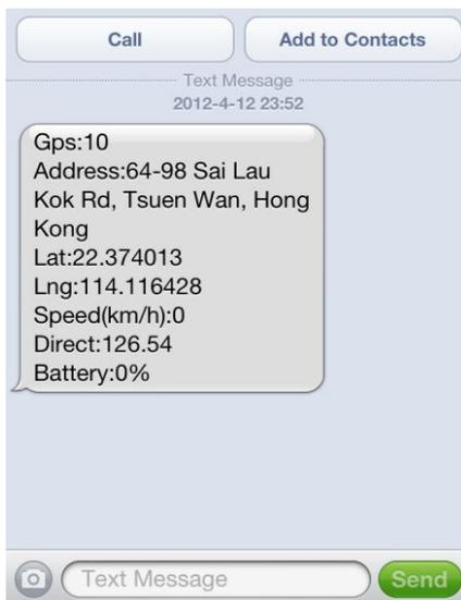
Send SMS "LOCATE\*123456" to the tracker, "LOCATE" is a command, "123456" is password. If the operation is success, the tracker will send back the information as above.
