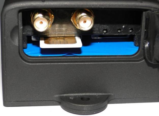
3.2 Please make sure that the SIM card is GSM network and able to execute the function of incoming calls display, no calls can be diverted and the PIN code is locked. The SMS format must be TXT format, and can't recognize the PDU format.
