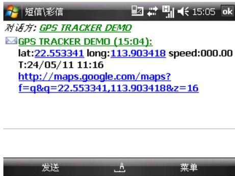
\*Tracking location, when no GPS signal, the SMS includes the last valid latitude & longitude as well as the LAC code of current position, the LAC code can be input in the column of “manual track” menu of web platform.
